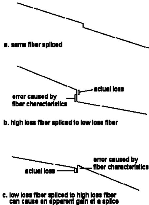
Figure 7. Loss errors in OTDR measurements
